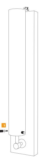
Connect wires from fixture with provided wire nuts to electrical box.
