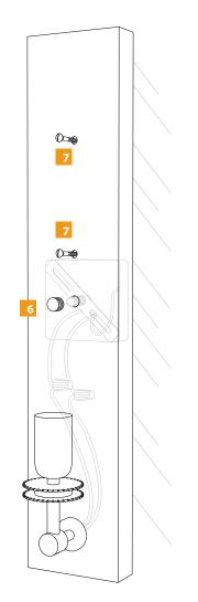
8 Screw in provided screws into anchors, DO NOT OVER TIGHTEN
