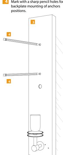
Screw in provided heavy duty Self tapping EZ anchors.
